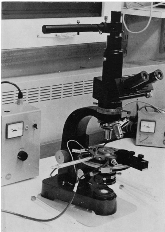
**Figure 3** (Top left). The Microscope Room, detail of microscope bench. The Leitz Ortholux microscope occupies the central position. Connected to the phototube at the top is the 35mm. Orthomat camera, its control box on the bench far right. The large-format camera, with ground glass screen for focusing the image, has been slid up the vertical support out of the way, its control box being on the shelf adjacent.
