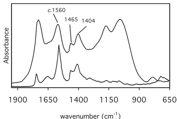
FIG. 1 Infrared spectra (1950–650  $\text{cm}^{-1}$ ) of: (1) smalt test film exposed to heat and light (upper trace); (2) a standard sample of potassium soaps (prepared by adding KOH to fresh linseed oil, lower trace).
