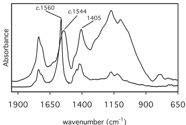
FIG. 2 Infrared spectra (1950–650  $\text{cm}^{-1}$ ) of: (1) smalt test film over lead white priming exposed to light at 90% RH (upper trace); (2) methanol extractables from the same film (lower trace).
