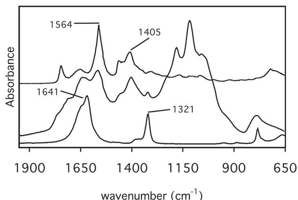
FIG. 3 Infrared spectra (1950–650  $\text{cm}^{-1}$ ) of: (1) a standard sample of potassium soaps (prepared by adding KOH to fresh linseed oil, upper trace); (2) smalt test film prepared by Plesters in 1964 and subsequently aged naturally (middle trace); (3) a standard sample of calcium oxalate prepared in the laboratory (lower trace).
