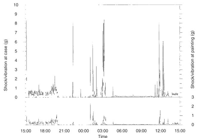
**Fig. 5** Shock/vibration record for part of the transportation from the Chrysler Museum, Norfolk, Virginia to the National Gallery: the upper trace is from the logger attached to the case, the lower trace is from the logger attached to the painting.
