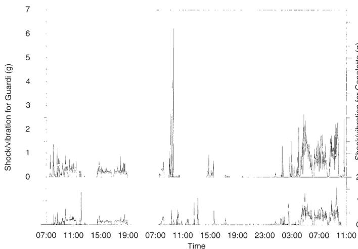
**Fig. 6** Shock/vibration record for part of the transportation from the Royal Academy, London, to the National Gallery of Art, Washington: the upper trace is from the logger attached to Guardi's *An Architectural Caprice with a Palladian Style Building* (NG 2517), the lower trace is from the logger attached to Canaletto's *Venice: The Feast Day of Saint Roch* (NG 937). Note the discontinuity in the time axis during the first overnight period.
