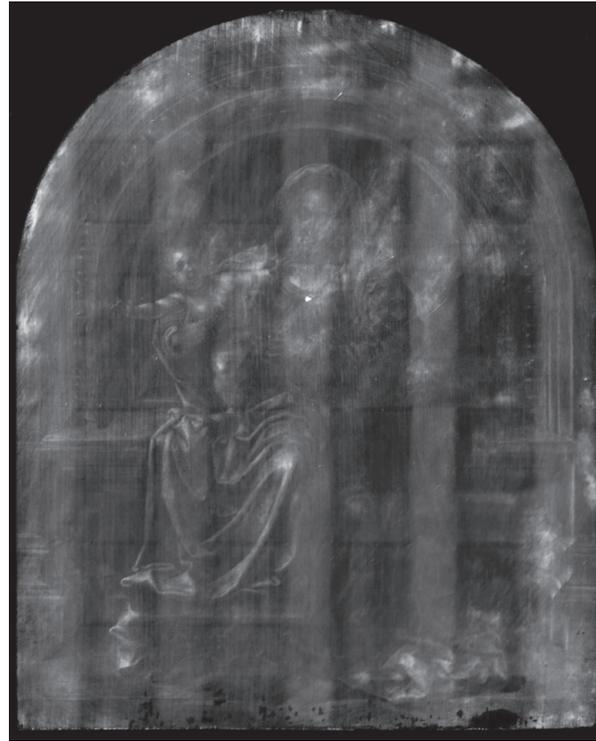
b. Equivalent radiograph made while the painting was moving with respect to the X-ray source.
