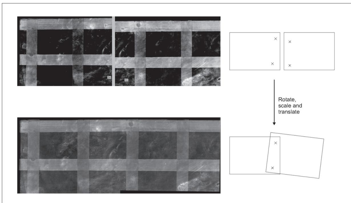
FIG. 2 Schematic showing the use of two tie points in each image to scale, rotate and translate an image during mosaic assembly; the line diagram to the right somewhat exaggerates the magnitude of the rotation and scaling required for the image pair to the left. Note that the slight difference in exposure between the two plates has not been corrected at this stage.
