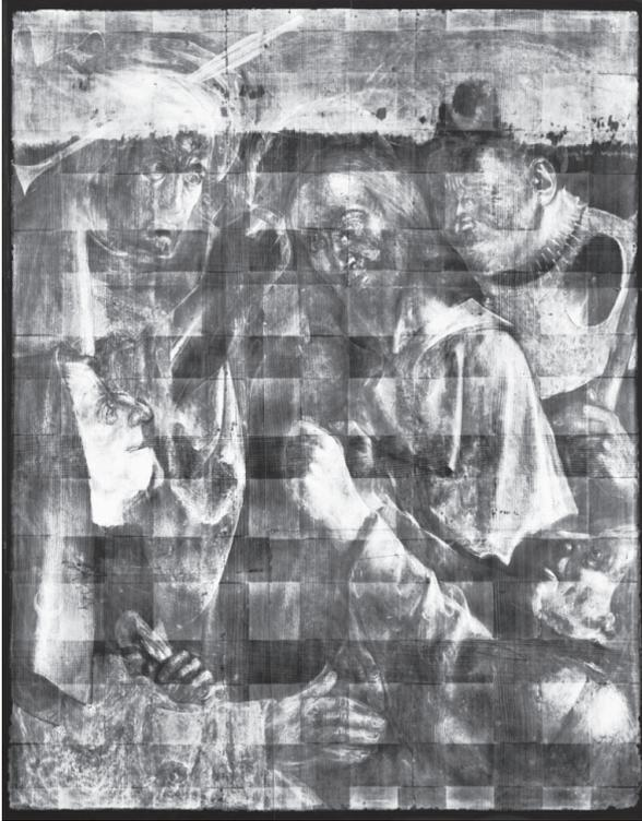
a. Traditional hand-assembled 'cut-and-paste' composite X-radiograph, re-photographed on black and white film.
