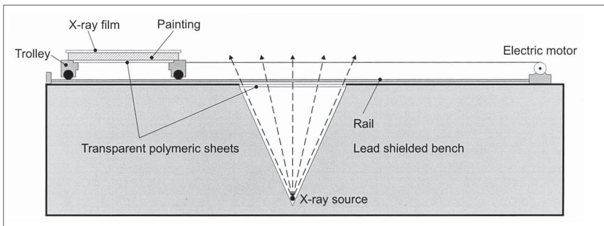
FIG. 8 The simple experimental set up used to acquire strati-radiographs at the National Gallery
