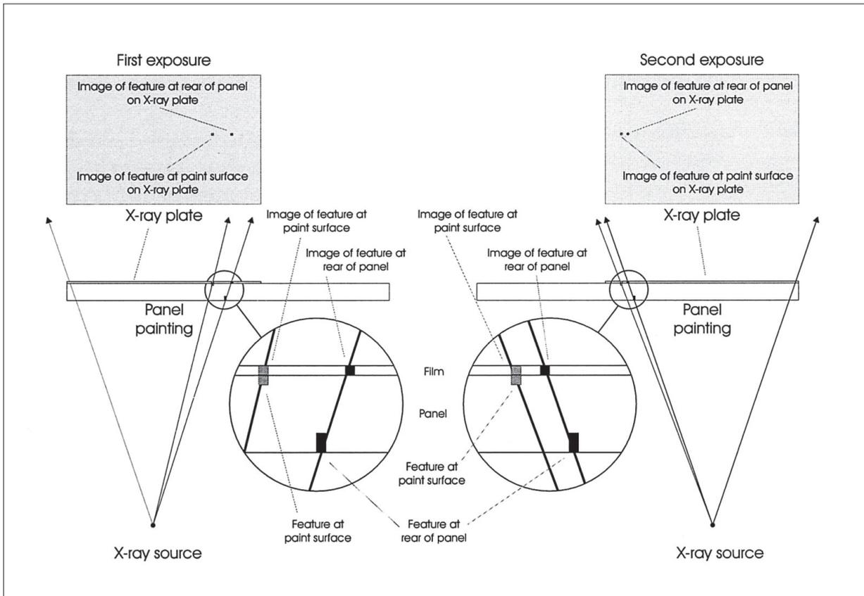
FIG. 3 The effect of diverging X-rays on the relative position in the images of features at different depths in the painting structure.
