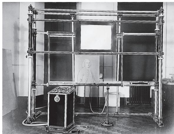
FIG. 1 The equipment used for X-radiography at the National Gallery during the 1930s.
