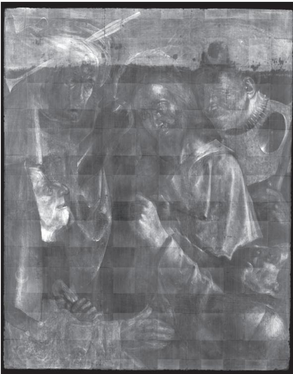
c. X-radiograph made by filling the interstices in the cradle with sugar.
