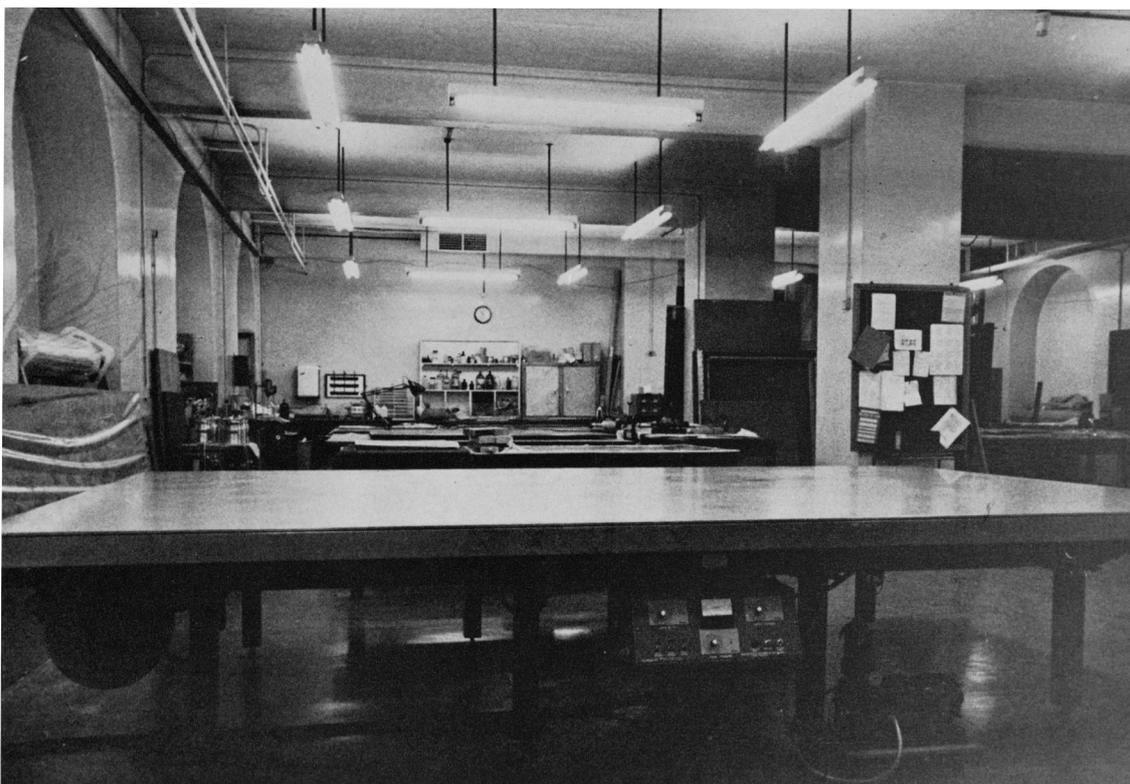
**Figure 7** The main Conservation Workshop looking north. The large vacuum hot-table (foreground) measures 4m×2.5m. The control panel incorporates separate controls for main and edge heaters and a safety cut-out overriding both. When not in use, the hot-table is covered and provides another work surface. The varnishing room and the lift serving the North Conservation Studio are beyond the doors just visible at the far right.
