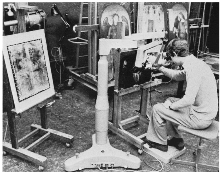
**Figure 3** Hydraulic easel and chair. This small hydraulic easel is designed to carry 150kg. The chair will rise to a seat height of 2.1m and has surfaces on either hand for solvents, paints and instruments.
