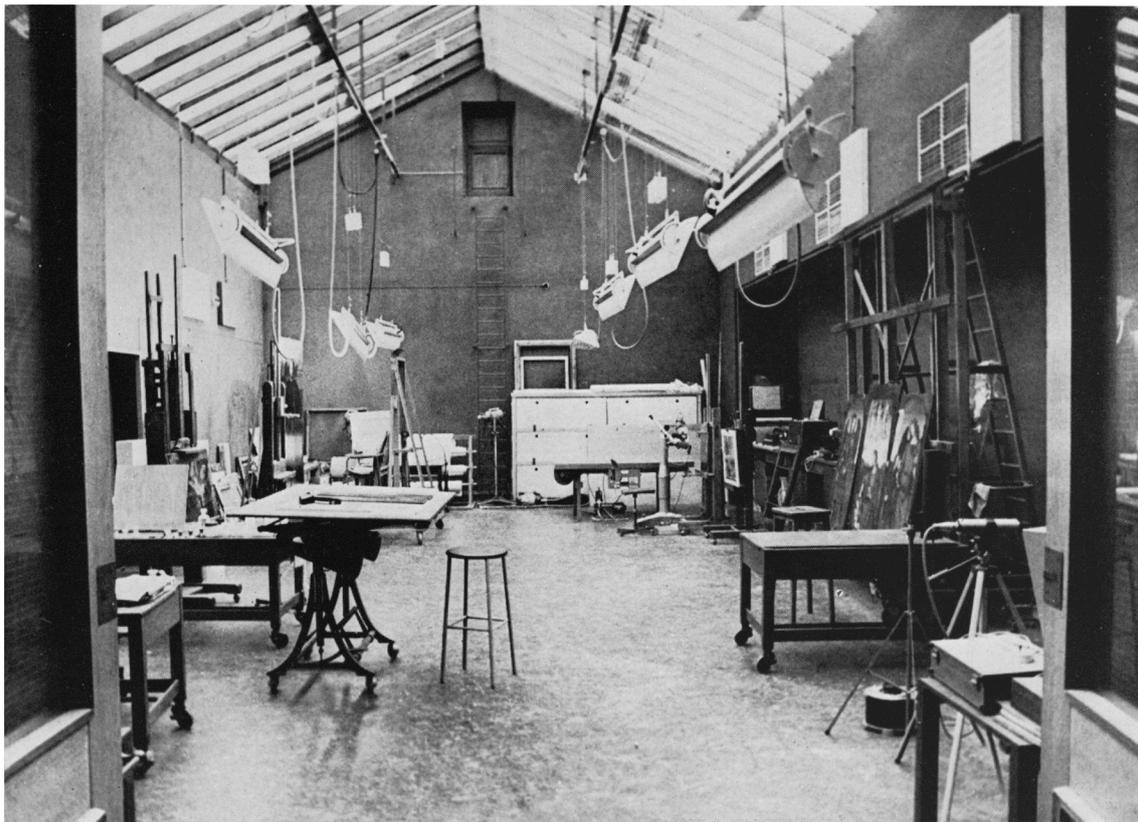
**Figure 1** The north Conservation Studio. The south-facing slope of the roof (right) has an internal system of venetian blinds. Banks of fluorescent lights are suspended, with counterweights, from tracks running the length of the studio. The large hydraulic easel (right) is capable of raising 750kg. The small vacuum hot-table (3m×1.2m) can be seen beyond the microscope at the far end.
