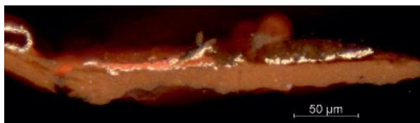
FIG. 9 NG 579, paint cross-section taken from the *sgraffito* on the right main tier panel (Saint Paul) showing water gilding over red bole. A vermilion paint layer is present on top of the gold leaf.
