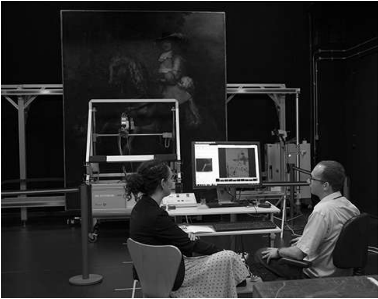
Nelly von Aderkas and David Peggie using the X-ray fluorescence (XRF) scanner to image the earlier composition beneath Rembrandt's Portrait of Frederick Rihel on Horseback (see pp. 44–6)
