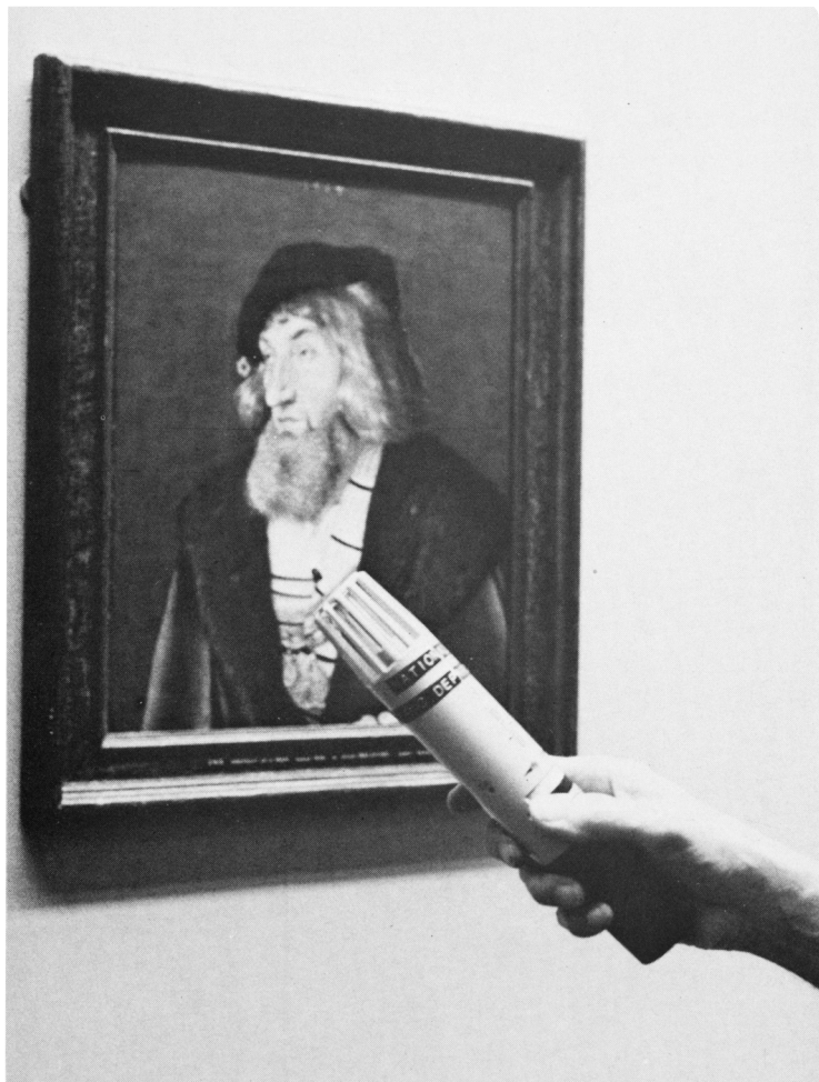
Figure 3 Hand-held self-calibrating electronic hygrometer (Nova Sina Mik 5317). This type of instrument is very much easier to use than the sling hygrometer, and its accuracy can be checked at any time by placing a special cap over the sensor at the top of the instrument. This cap provides a standard RH (55% in this case) against which the instrument can be corrected.
