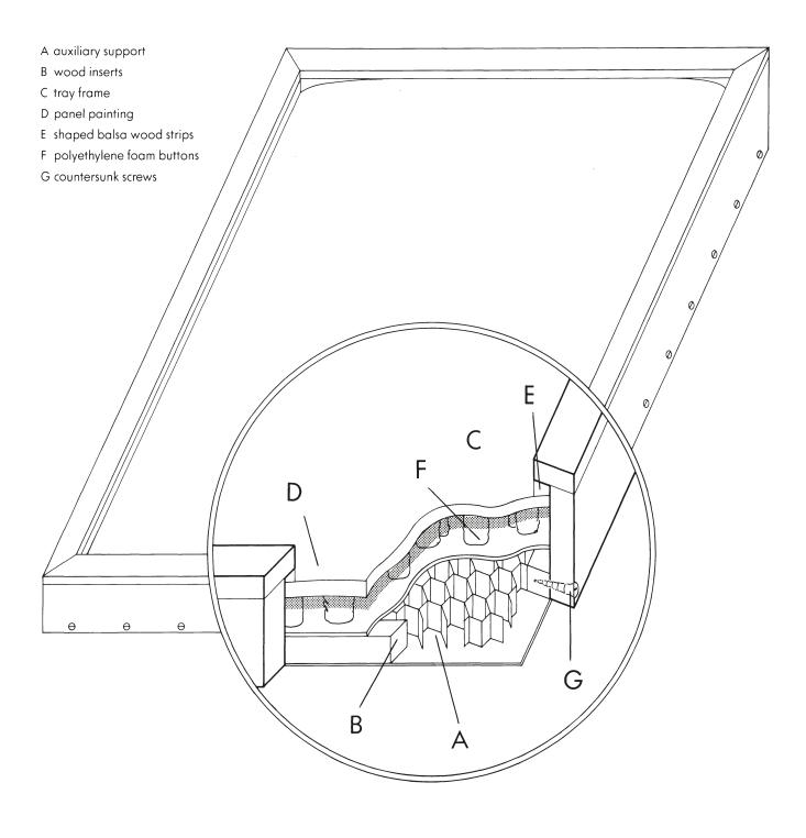
Figure 5 Cut-away diagram showing the structure of a panel tray.
