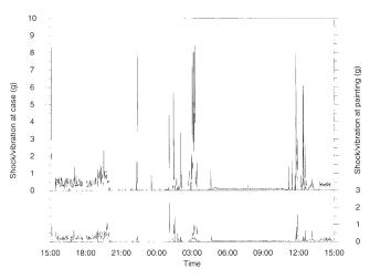
Fig. 5 Shock/vibration record for part of the transportation from the Chrysler Museum, Norfolk, Virginia to the National Gallery: the upper trace is from the logger attached to the case, the lower trace is from the logger attached to the painting.
