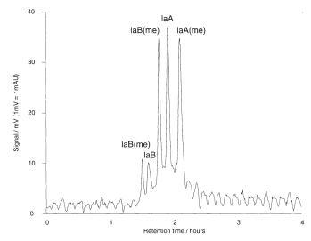
Fig. 1b Chromatogram of lac lake (prepared in the laboratory), after treatment with 5% boron trifluoride- methanol; laA, laB: laccaic acids A and B; laA(me), laB(me): methylated derivatives of laccaic acids A and B.
