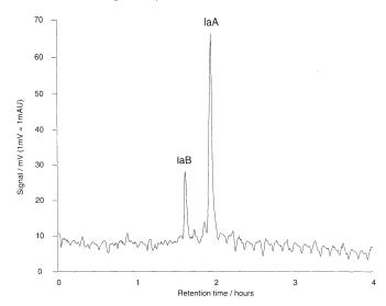
Fig. 1a Chromatogram of aqueous extract of lac dyestuff from stick lac (Kerria sp.); laA: laccaic acid A; laB: laccaic acid B. Eluents and conditions described in the text.
