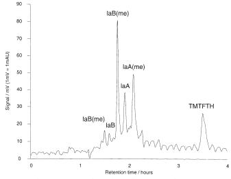
Fig. 1c Chromatogram of lac dyestuff extracted from sample of the red cloak, from Cardinal Richelieu (NG 1449), painted by Philippe de Champaigne, c.1637; after extraction of paint medium with TMTFTH, a trace of which has produced the peak thus labelled. Laccaic acids as before.
