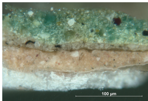
PLATE 3 Cross-section of a sample from the green shaded area of the Magdalen's dress. The green layer contains a copper green pigment, lead-tin yellow, lead white, yellow earth and a few large carbon black particles. The original mid-brownish grey imprimitura of lead white, a coarse carbon black, brown earth, and a little lead-tin yellow is visible under the green paint. All layers below this were added as part of the various transfer processes. The red ground layer is presumed to have been applied by Hacquin in the late eighteenth century, while the titanium white ground was added to the reverse in 1958.
