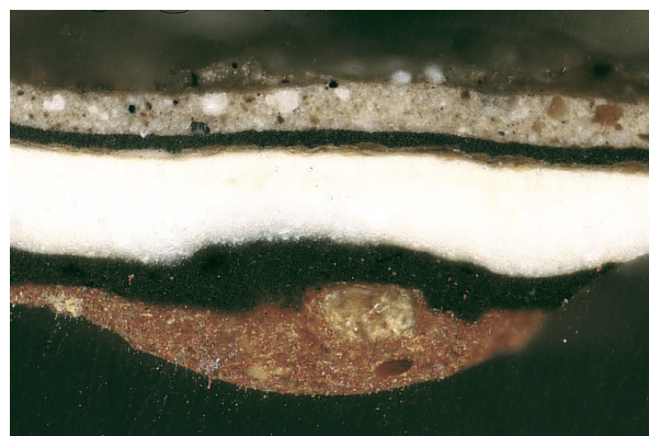
PLATE 3 Cross-section of a sample from the shields on the right wing. The thick, lead white, blocking-out layer is visible in the middle of the section on top of the black paint of the first shield. The black paint of the second shield lies over a thin, yellowish-brown proteinaceous layer which covers the white, and is in turn covered by several layers of brown paint. Original magnification 280x, actual magnification 240x.
