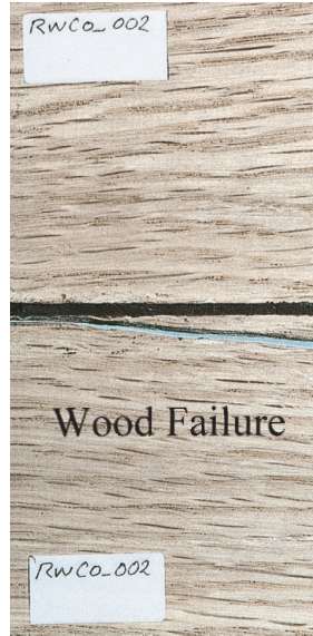
PLATE 5 Failed joint – Resin W/Coconut flour.
