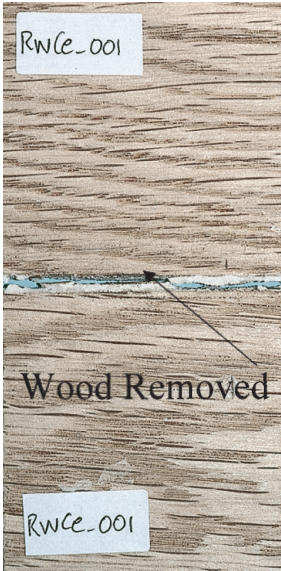
PLATE 4 Failed joint – Resin W/Cellulose powder.
