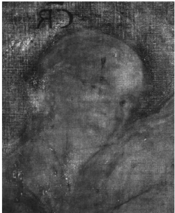
FIG. 183 NG 3, detail of transmitted infrared image, taken from the front of the canvas.
