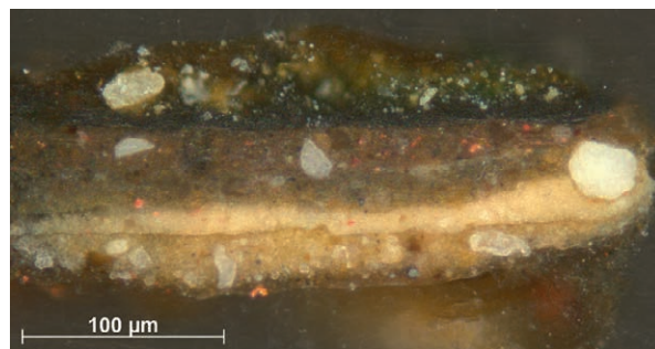
FIG. 190 NG 3, paint cross-section from the recorder player's green hat.
