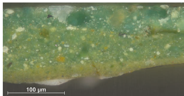
FIG. 97 NG 4, paint cross-section from the green foliage.
