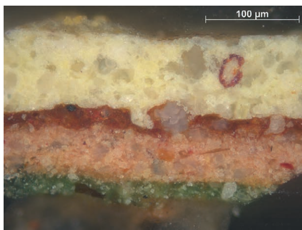
FIG. 64 The Flight into Egypt , paint cross-section from Joseph's yellow robe.
