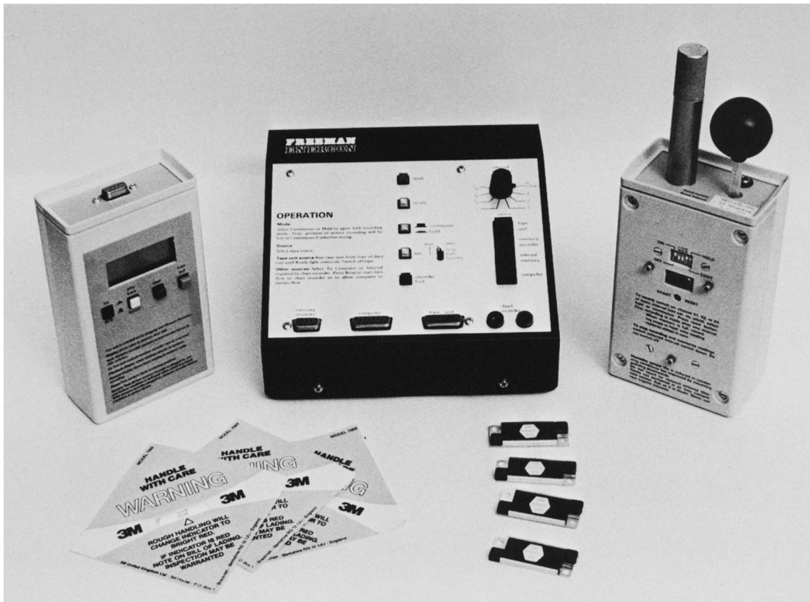
Figure 6 (Behind right) Freeman Enercon temperature- and RH- solid-state memory recorder. (Behind centre) Memory transfer unit to output readings from recorder to computer. (Behind left) Test/display unit to check function and battery of recorder. (Foreground right) Drop (N) Tell Impact Indicators. (Foreground left) 3M Shockwatch.
