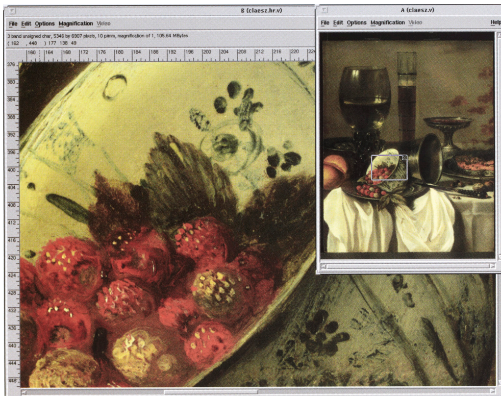
Plate 2 Selecting a detail. The low-resolution image at the upper right of the screen is used to select a detail from the high-resolution image. The remainder of the screen is occupied by the portion of the high-resolution image thus selected.
