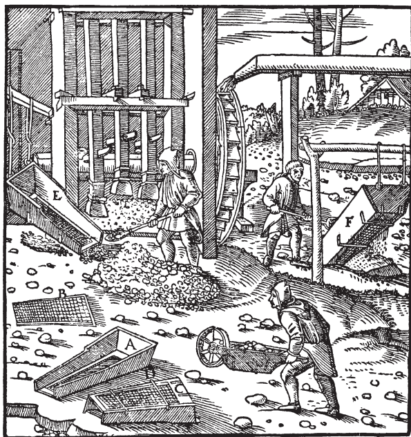
Fig. 1 Crushing and preliminary sieving of ore, from Georgius Agricola, De re metallica , Basel 1556. Letters A–F refer to the box-shaped sieve and its use.
