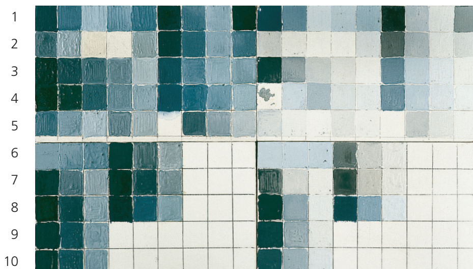
PLATE 12 Test samples of modern and historic Prussian blues, mixed with different proportions of lead white in oil medium, before (left) and after (right) exposure to light: see TABLE 1 for reference and shade codes. The sequence is identical for the faded panels on the right.
