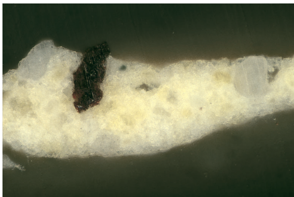
PLATE 8 Meindert Hobbema, The Avenue at Middelbarnis (NG 830), 1689. Cross-section from the lead-tin yellow highlight of the small tree in sunlight, showing relatively homogeneous inclusions. Original magnification 500x; actual magnification 440x.
