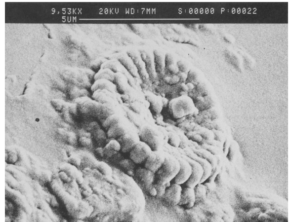
Figure 19 Martin van Heemskerck, The Donor and Saint Mary Magdalene . SEM micrograph showing a coccolith in the chalk ground. Gold-coated, 9530 \times .
