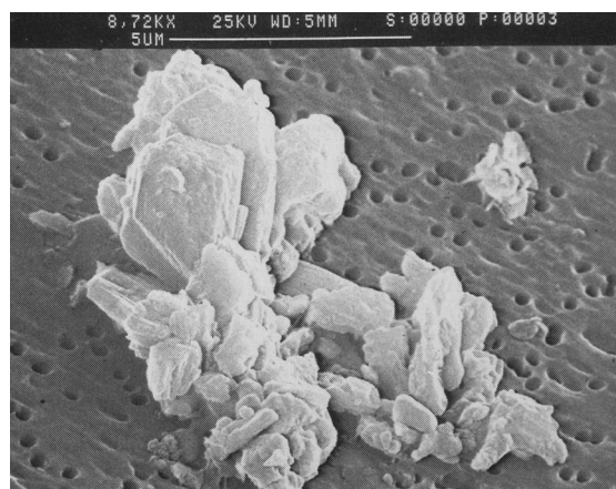
Figure 20 Samuel van Hoogstraten, the Peepshow . SEM micrograph of a sample of vermilion, probably of the dry process form. Gold-coated, 8720 ×.
