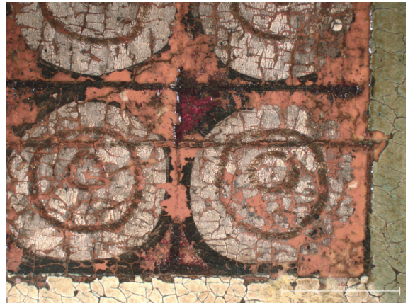
PLATE 20 Saint Francis before the Pope (PLATE 4), photomicrograph of central window, showing paint over silver leaf to depict glass roundels.
