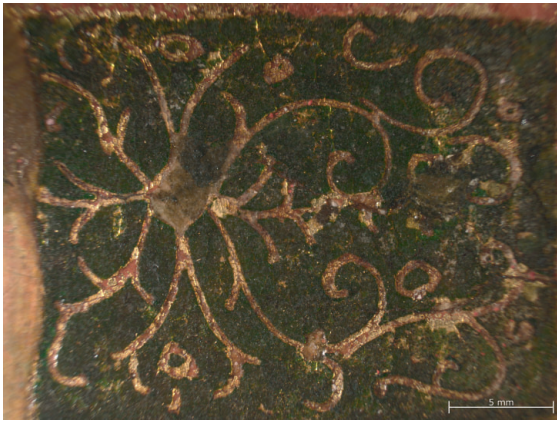
PLATE 17 The Funeral of Saint Francis (PLATE 8), photomicrograph of green sgraffito decoration on altarpiece.
