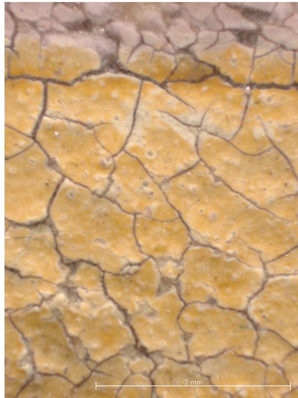
PLATE 39 The Funeral of Saint Francis (PLATE 8), photomicrograph of yellow marbling in architecture, showing lead soap pustules.
