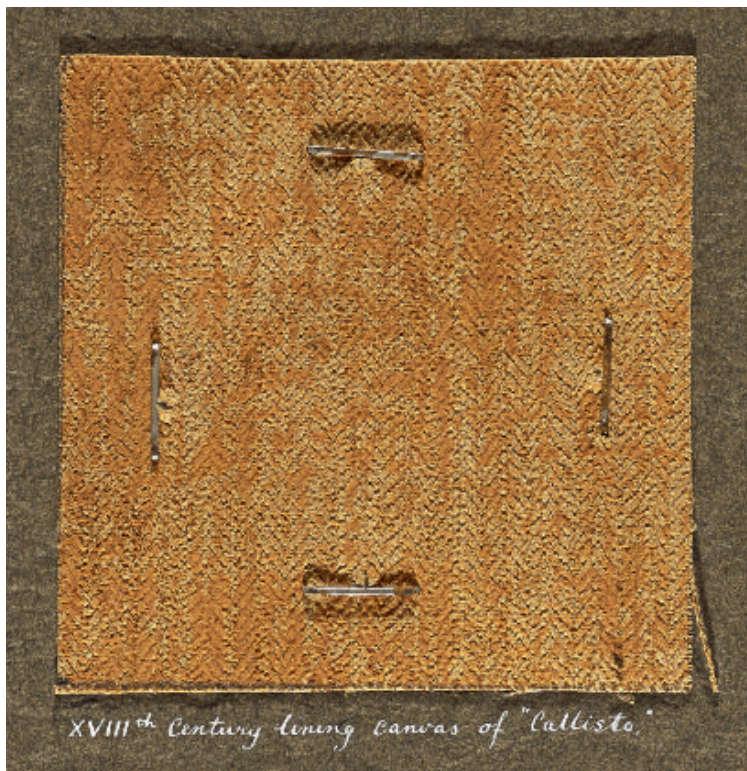
FIG. 250 A piece of the herringbone weave lining canvas removed from Diana and Callisto in 1932 and included in Kennedy North's documentation. He records the thread count as 48 × 68 to the inch.
