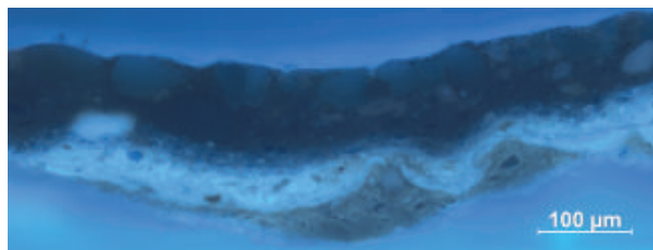
FIG. 148 NG 6611, NGS 2839, paint cross-section from the brighter green of the trees on the wooded slope in the middle distance, below the white buildings, under ultraviolet illumination.
