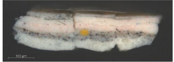
FIG. 173 *Frances, Countess of Lincoln*, paint cross-section from sleeve.
