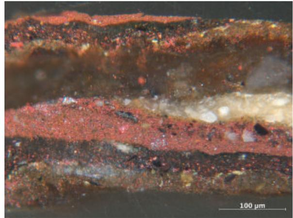
FIG. 176 *Colonel Tarleton*, paint cross-section from the background at the left edge.
