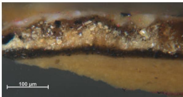
FIG. 178 *Colonel Tarleton*, paint cross-section from the yellow-brown drapery in the lower left corner, containing orpiment and other yellow pigments.
