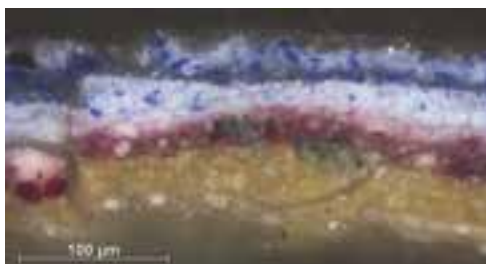
4 Paint cross-section from Titian's Bacchus and Ariadne , 1520–3 (NG35), showing reworking and overlap of paint layers created in the course of execution. Lapis lazuli (ultramarine) layers lie at the surface.
