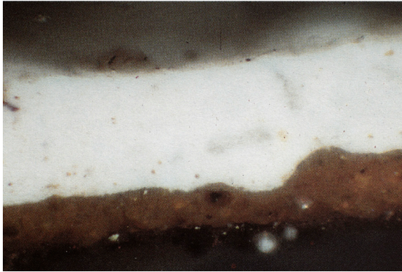
Plate 2 Cross-section from the turnover showing the double ground: a light grey preparation of lead white with some charcoal over a lower ochreous layer. Photographed under the microscope in reflected light at 275 \times ; actual magnification on the printed page 260 \times .
