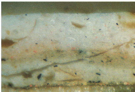
Plate 3 Cross-section from pinkish highlight on the Child's thigh. A very thin imprimatura over the chalk ground is just discernible, with some drawing. Over this are two blocking-in paint layers: the first of grey and the second of a warmer grey-brown. The flesh highlight comprises two further layers of lead white tinted with a little vermilion. Photographed in reflected light under the microscope at 510 \times ; actual magnification on the printed page 415 \times .
