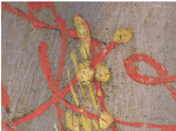
FIG. 7 NG 3927, photomicrograph detail showing the embroidered pattern on the angel's sleeve. The red is vermilion, and the yellow contains lead-tin-antimony yellow.
